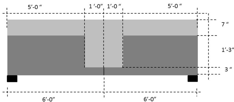
Fig. 13 Test specimen with a straight web profile. Width of the specimen is 4 ft - 0 in.
