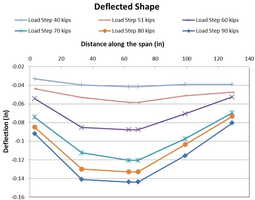
Fig. 24 Deflected shape of the specimen with the tapered web and no physical connection between the precast components and the cast-in-place topping for various load steps
