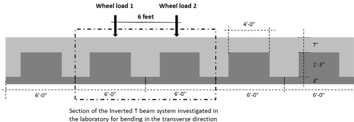
Fig. 10 This figure illustrates the rationale behind the selection of the geometry of the test specimens to investigate the performance of different connections and cross-sectional shapes when subject to bending in the transverse direction.
