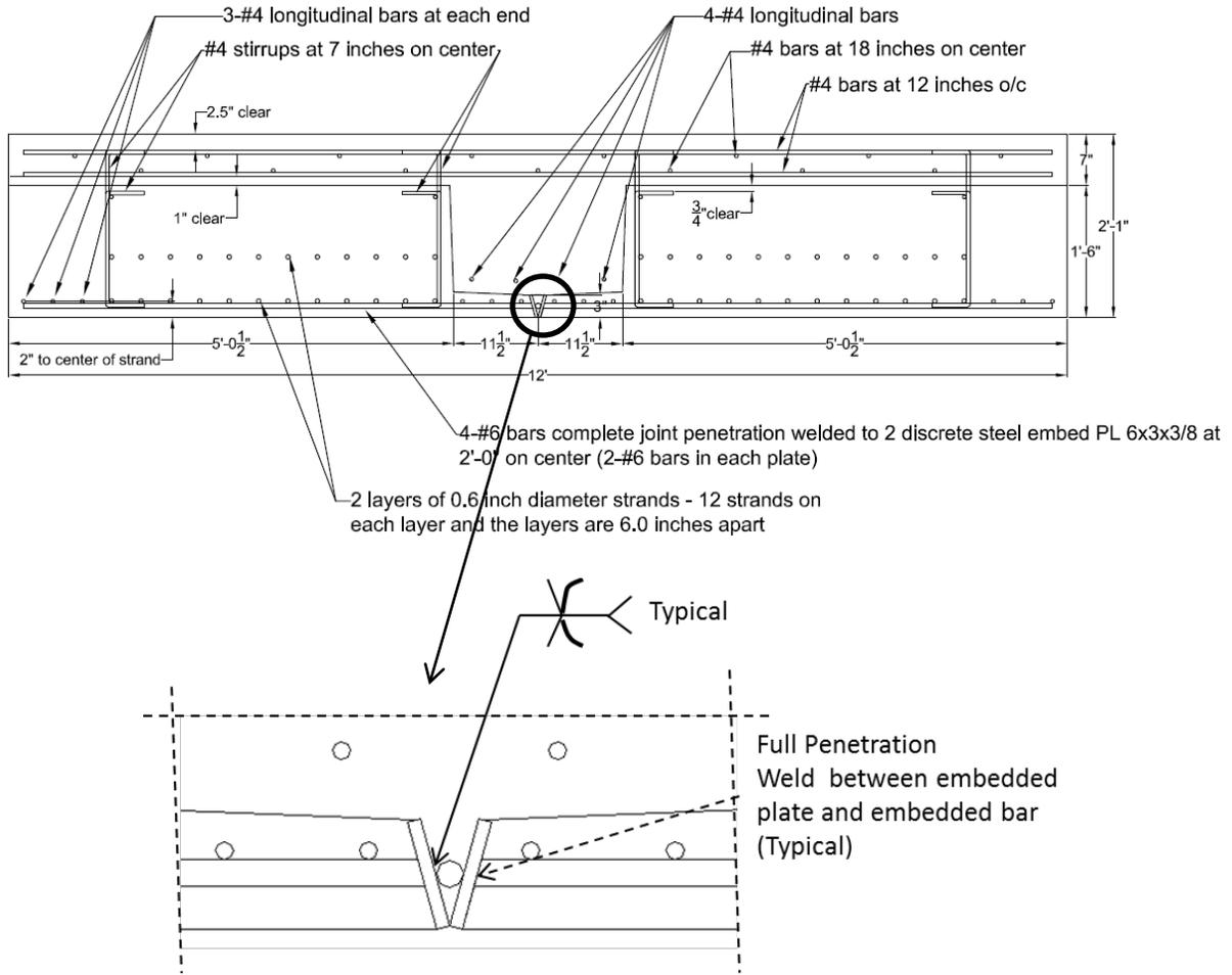
Fig. 16 Reinforcing Details for Test Specimen #2 – Straight web cross-sectional shape with embed plate connection
