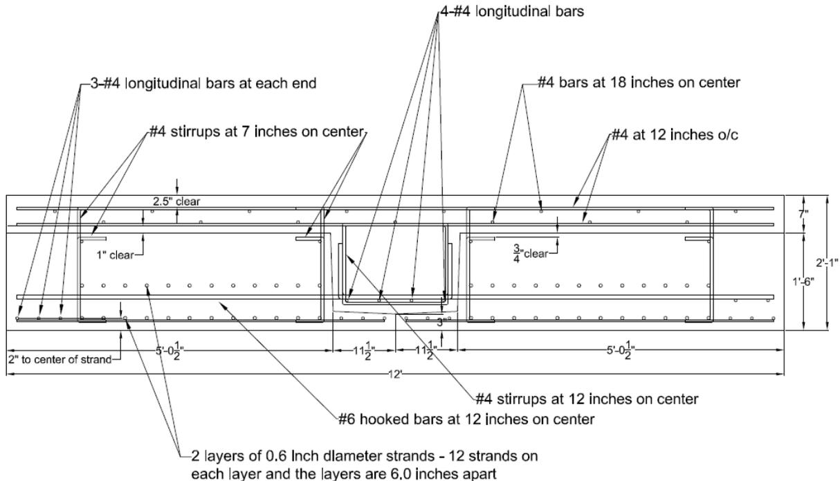
Fig. 15 Reinforcing Details for Test Specimen #1 – Straight web cross-sectional shape with extended bars
