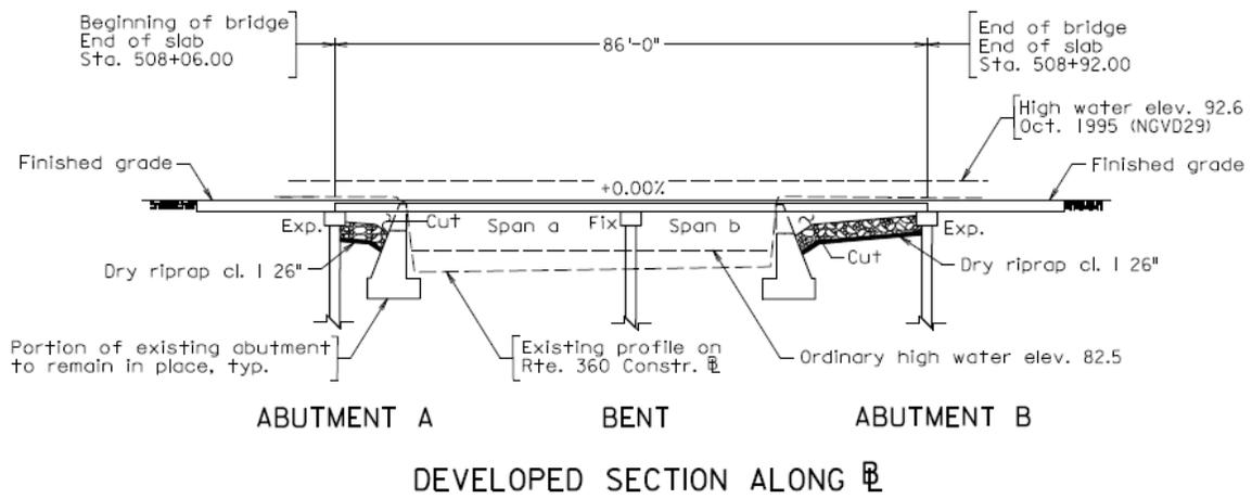
Fig. 6 Preliminary elevation of the soon to be replaced two-span continuous bridge on Route 360 over Chickahominy River (Courtesy of Virginia Department of Transportation<sup>6</sup>)
