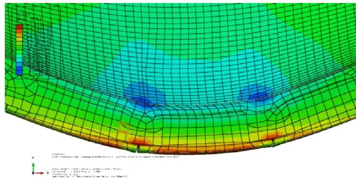
Fig. 9 A sectional cut in the transverse directions to illustrate maximum transverse flexural stresses above the joint between the precast inverted T-beams
