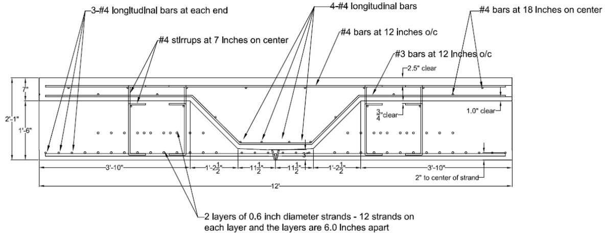
Fig. 17 Reinforcing Details for Test Specimen #3 – Tapered web cross-sectional shape with embed plate connection
