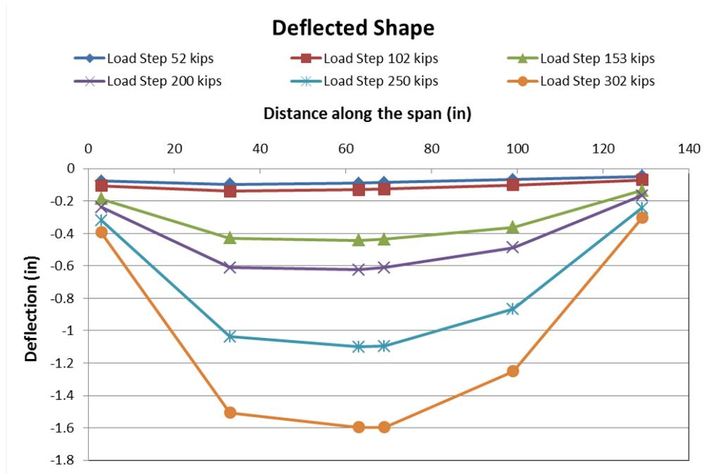
Fig. 22 Deflected shape of the specimen with tapered web and embedded plate connection for various load steps
