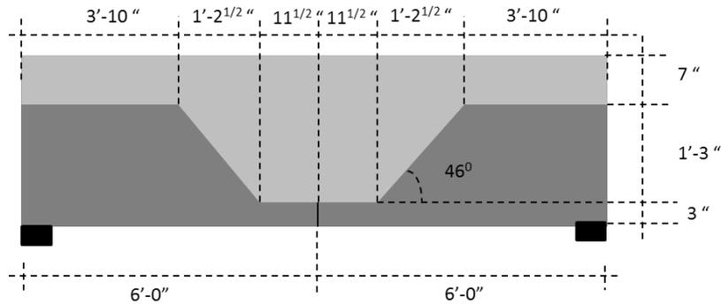
Fig. 14 Test specimen with a tapered web profile Width of the specimen is 4 ft- 0 in.
