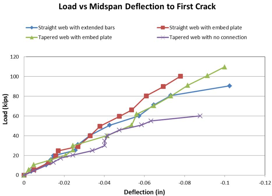
Fig. 20 Comparison of Load Deflection Curves for all four specimens up approximately first crack.
